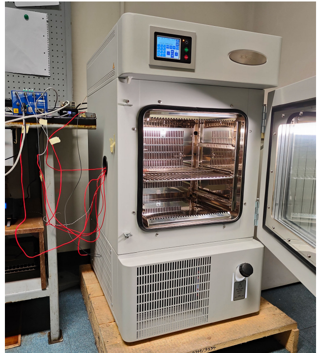
FIGURE 9. The setting used to conduct temperature measurement test. It is possible to see the climatic chamber containing the sensors network.
