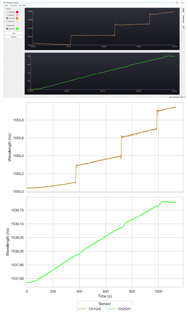
FIGURE 11. A comparison between the Measures view of the PhotoNext FBG Data Analyzer during simultaneous strain (in brown for the selected sensor) and temperature measurement (in green) test and post-processing analysis made on data saved on the Cloud Database .
