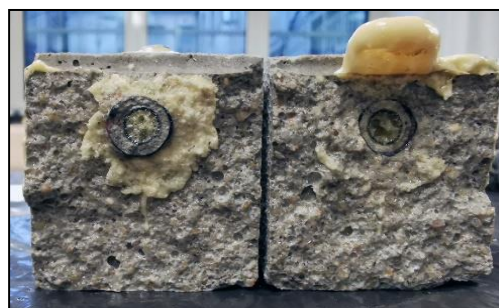
Fig. 1. Cross-section of a PUC specimen after failure showcasing the ruptured resin capsule and the spilled resin.
