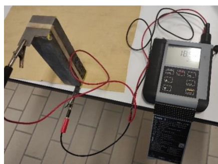
Fig. 3. Set up for electrical conductance measurements.
