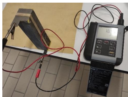
Fig. 3. Set up for electrical conductance measurements.
