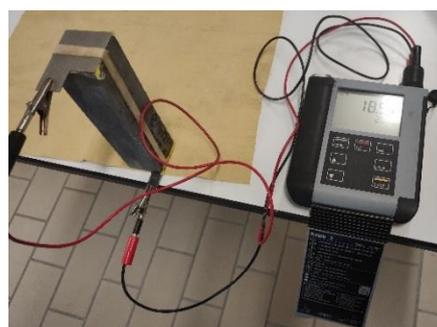
**Fig. 3.** Set up for electrical conductance measurements.
