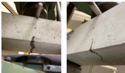
Fig. 5. Successful rupture of embedded capsules by releasing the sealing agent through the crack
