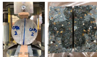
Fig. 9. Splitting the cylindrical specimens to count the amount of broken capsules in a certain crack plane (note: the darkest concrete surface is the area covered by WRA)
