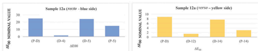
Figure 4. \Delta E_{00} of the various treatment levels of the sample 12a (blue side and yellow side). P: before any treatment (level 0). D: after artificial ageing and soiling (level 1). 1; 2; 3 ...: laser-treated areas (level 2, Table 3).
