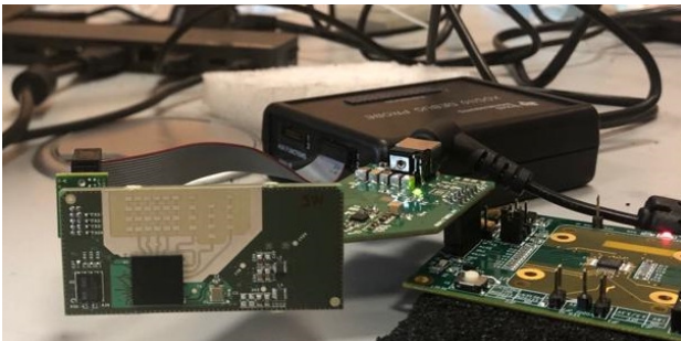
Fig. 10: Realized Radar board prototype
