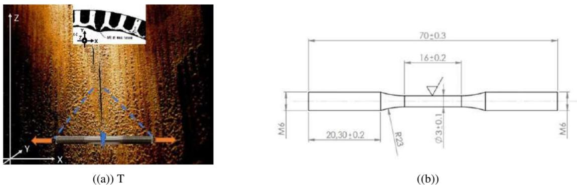
Figure 6: a) typical LRE z-axisymmetric plane fracture.<sup>6</sup> b) Low cycle fatigue and creep tests specimen geometry.
