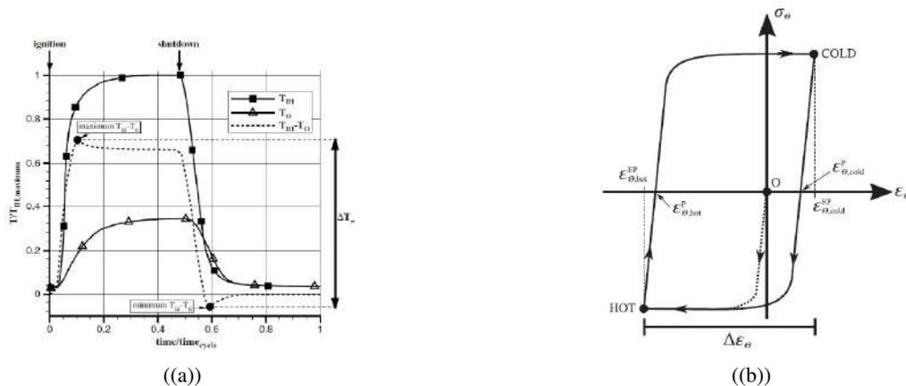
Figure 2: a) Typical behavior of the hot-gas-side ( $T_{IH}$ , squared dots) and backside wall temperatures ( $T_o$ , triangular dots) and their difference for a regeneratively cooled thrust chamber (dotted line).<sup>15</sup> b) Common cyclic stress-strain behavior of the hot-gas-side wall for a regeneratively cooled thrust chamber<sup>15</sup>
