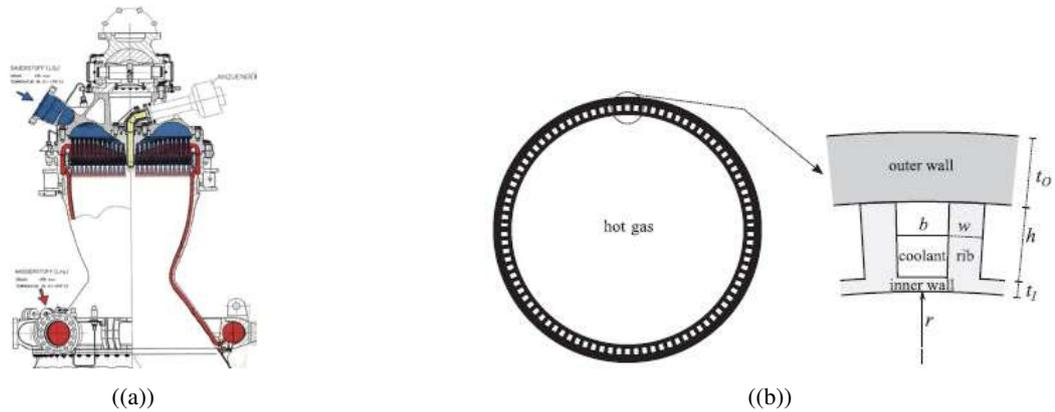
Figure 1: a) Schematic representation of the Vulcan thrust chamber assembly system.<sup>6</sup> b) Schematic of a regenerative thrust chamber cross section<sup>15</sup>
