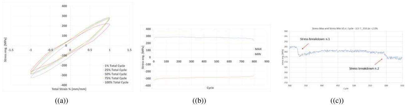
Figure 17:  $350^{\circ}\text{C}$  temperature LCF test at  $\Delta\varepsilon = 2.0\%$ . a) Cycles at different cycle to failure steps. b) Maximum and minimum stresses to failure. c) Stress breakdown effect.
