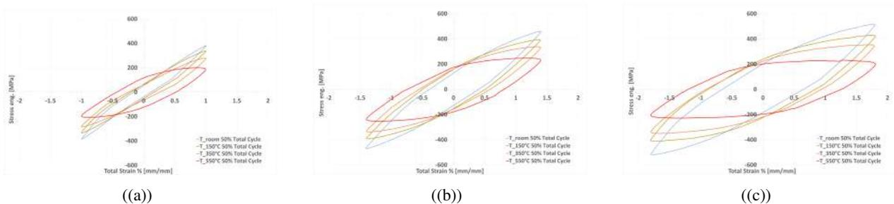
Figure 12: Low Cycle Fatigue temperature effect at constant strain. a)  $\Delta\varepsilon_{tot} = 2.0\%$  at 50% of total cycles vs Temperature. b)  $\Delta\varepsilon_{tot} = 2.8\%$  at 50% of total cycles vs Temperature. c)  $\Delta\varepsilon_{tot} = 3.6\%$  at 50% of total cycles vs Temperature.
