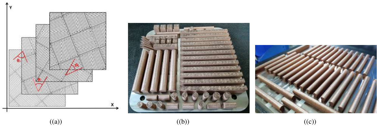
Figure 5: Additive Manufacturing scanning strategy and job layout. a) Layer random island strategy. b) Printing Job number 1 with cube specimens for micrography analysis at the top left corner of the platform. c) Printing Job number 2 with low cycle fatigue and creep row cylinders before machining.
