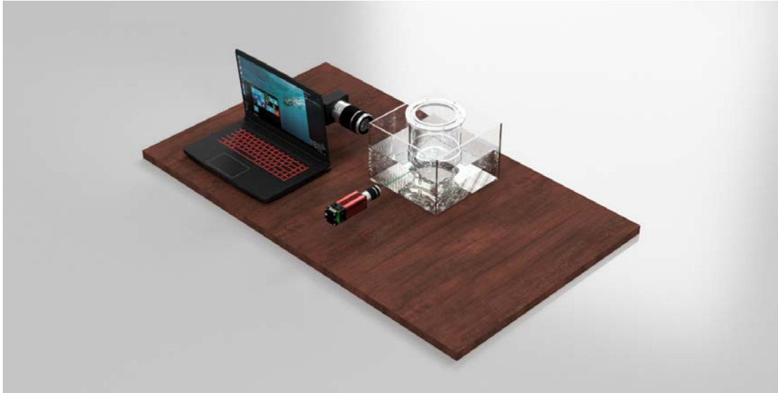
Figure 2: PIV system and the bioreactor configuration for images acquisition employed during this work. The Suspence® bioreactor was positioned inside a glass tank filled with distilled water to reduce refractive and diffractive light phenomena. A green laser and a camera (Dantec Dynamics, Denmark), positioned perpendicularly to the laser beam, were also used.
