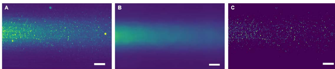
Figure 9: Effect of the background noise removal filter on PIV images of NPs-SCHO within SUSPENCE®. (A) Non filtered PIV image (B) PIV image containing only the background noise and (C) Filtered PIV image using Python script. Analysed section number: 3. Scale bar = 5mm.
