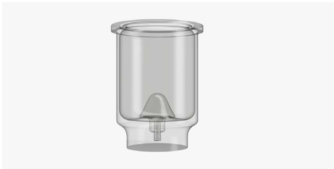
Figure 1: 3D rendering of the inner geometry of the vessel of Suspence® bioreactor. Cells are seeded inside the vessel and they move from the bottom part to the top.
