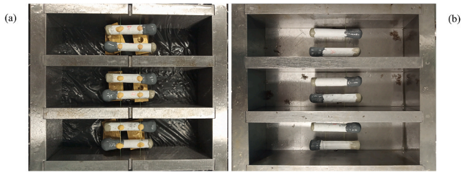
Fig. 3. (a) Placement of macrocapsules in moulds – bottom view (b) Placement of macrocapsules in moulds – top view.
