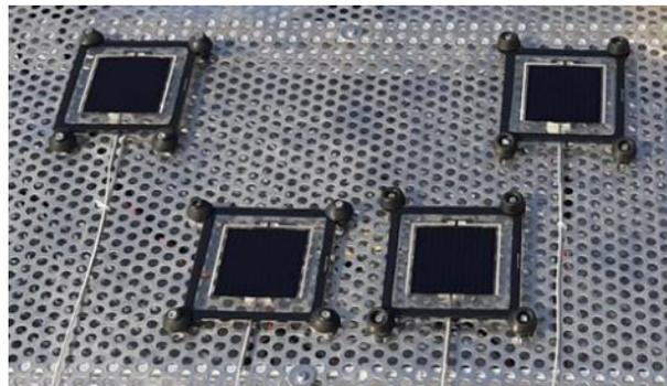
Fig. 4. PSCs under test.
