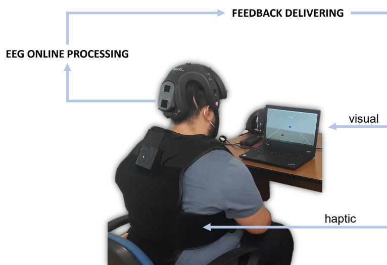
Figure 1. A subject using the proposed BCI system with neurofeedback in extended reality. The system involves EEG acquisition with the Helmata device, online processing, and actuators for visual–haptic feedback delivery.
