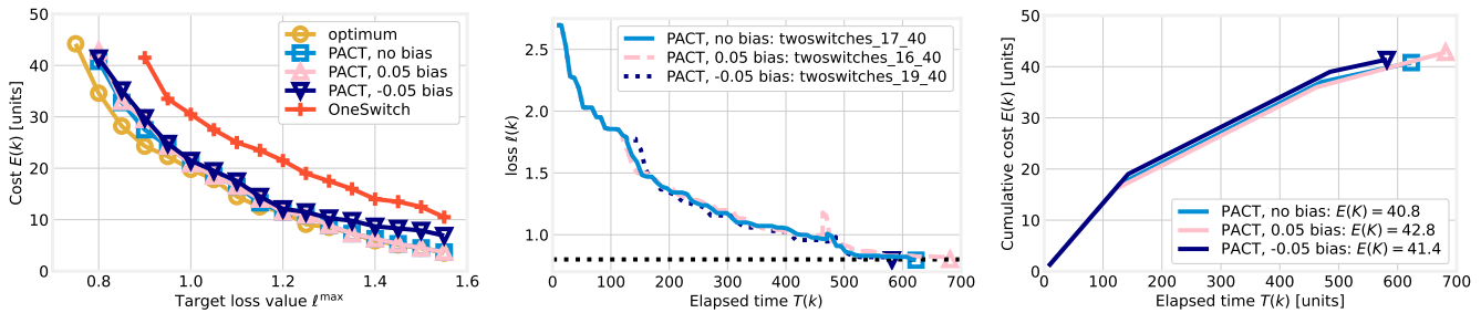
Fig. 14. Impact of quality of \hat{\lambda}^{\text{run}} for sequential scenario with AlexNet: PACT’s energy cost for different values of \ell^{\max} (left); loss (center) and cost (right) evolution for \ell^{\max} = 0.8 .
