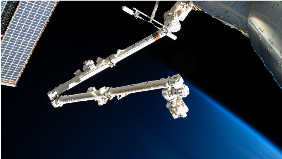
Fig. 1.1 The International Space Station's 57.7-foot-long robotic arm, also known as the Canadarm2, is pictured attached to the Harmony module as the orbital complex flies into an orbital sunrise above the Pacific Ocean. (credit: NASA)
