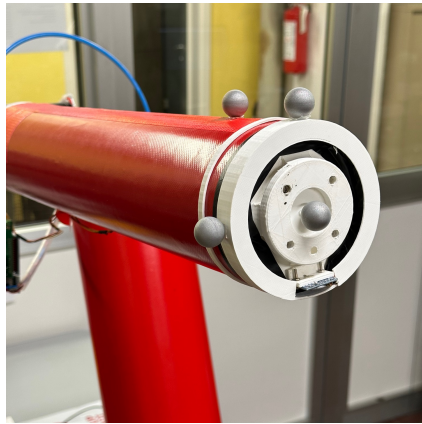
Fig. 3.26 OptiTrack Markers mounted on the robot flange
