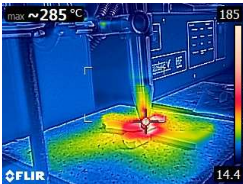
Figure 6-6: Thermal image of APPJ treatment on C/SiC (after 10 min of treatment).
