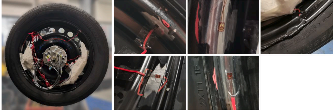
Fig. 16. Experimental setup on MTS 855 biaxial fatigue test bench.
