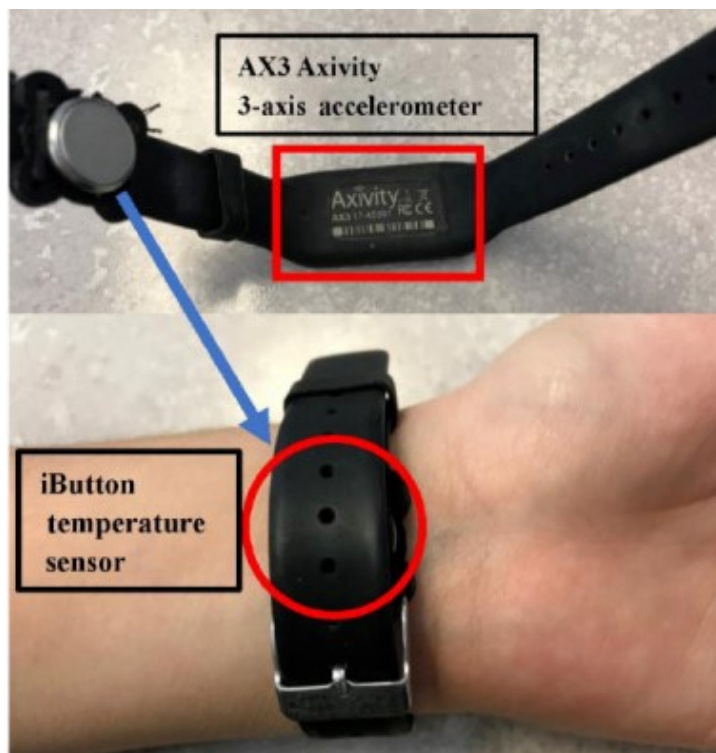
Figure 6. Custom-built wristband for actigraphy and temperature measures, employed for sleep quality assessment. The figure is adapted from [108].
