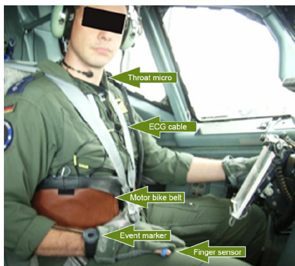
Figure 4. Instrumentation setup employed and shown in [76] for real-time monitoring. The authors registered a single-lead ECG, finger temperature, pulse wave, and EDA.
