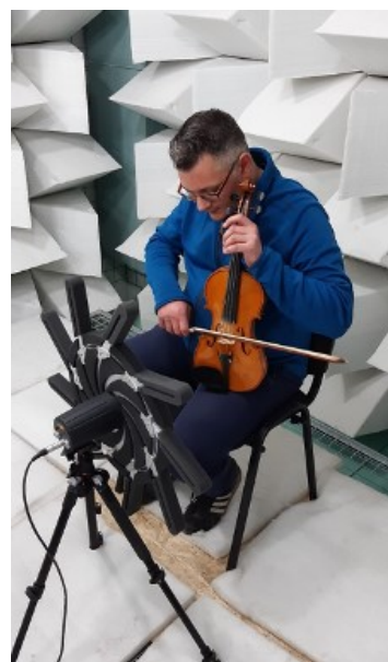
Figure 2. Experimental set-up for the identification of sonic sources.
