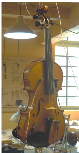
Figure 1. Set-up for the Modal Experimental Analysis.
