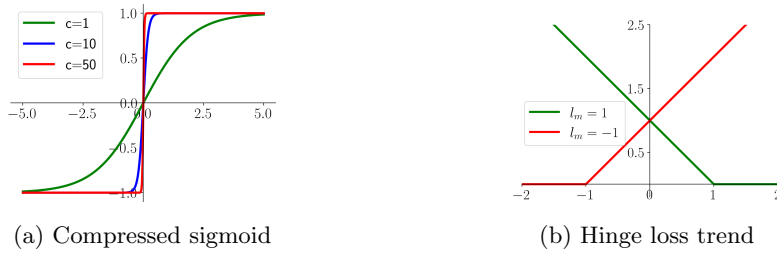
Fig. 2: (a) Increasing c in the MSE compressed sigmoid transforms it into a Heaviside step function: the loss is zero when the output score has the correct sign. (b) H loss trend for positive ( l_m = 1 ) and negative ( l_m = -1 ) pairs ( \delta = 1 ).
