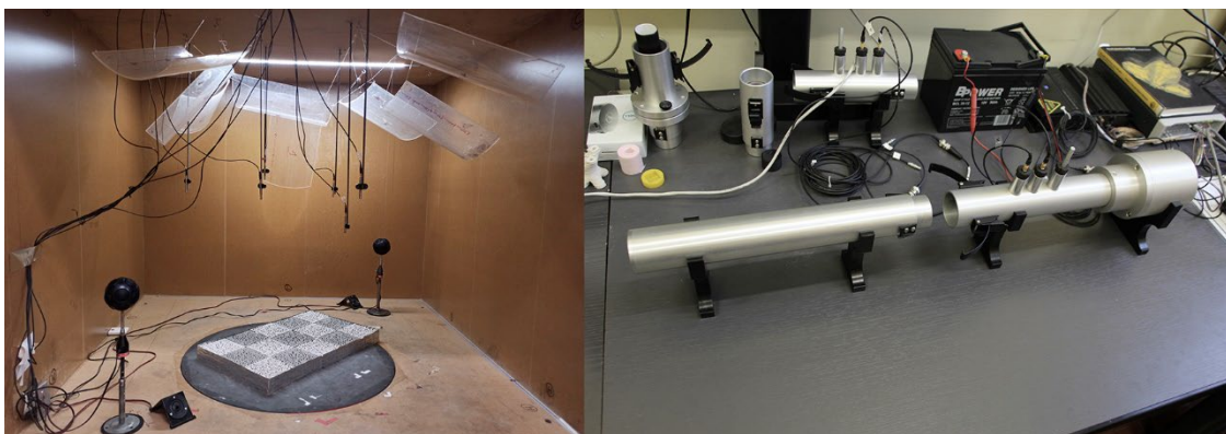
Figure 6. Left) Reverberation Chamber; Right) Impedance Tube.
