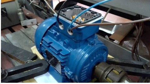
Fig. 2. The 550W TENV induction motor.
