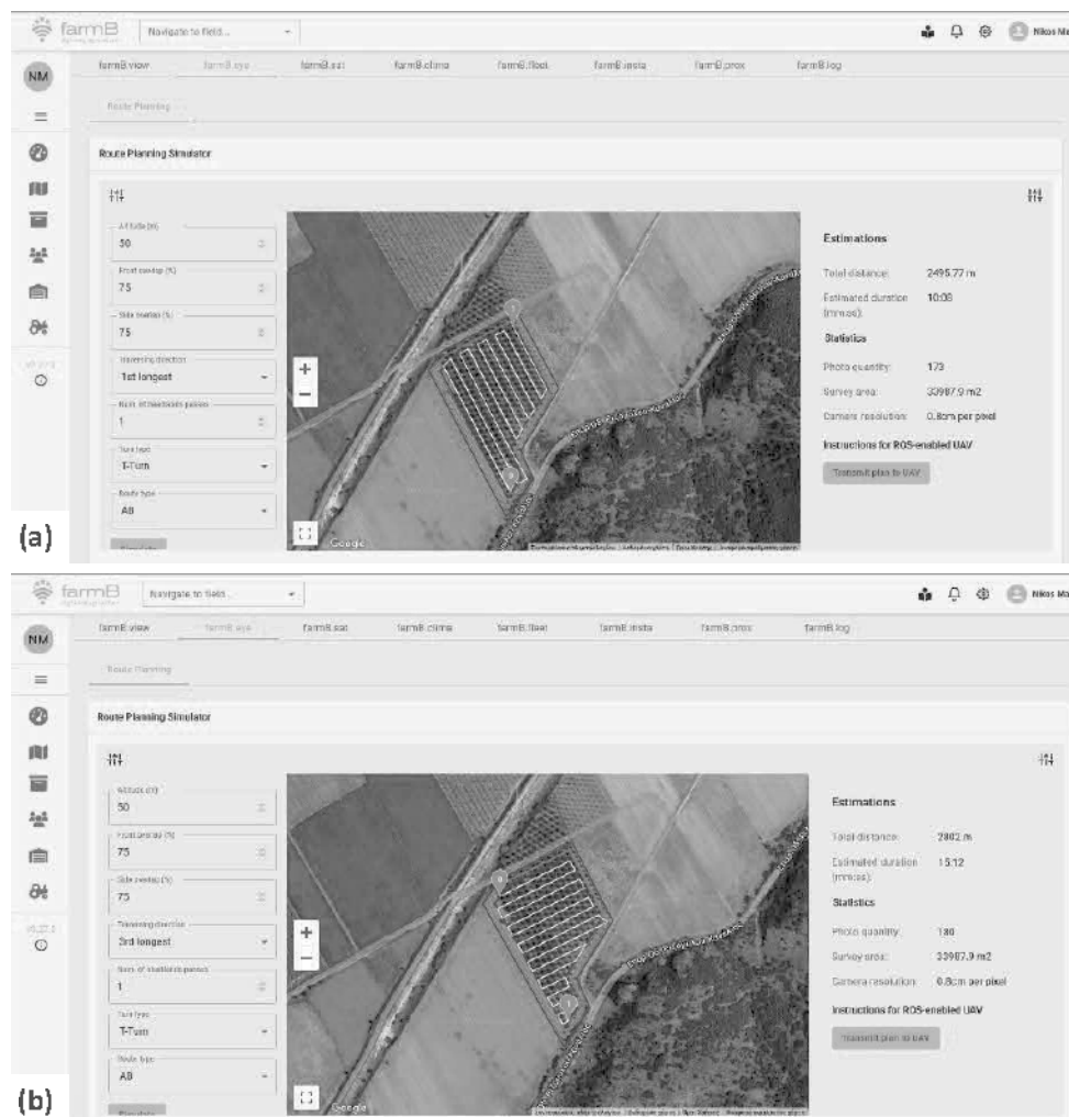
Figure 3. The FMIS digital platform interface for the generation of the UAV area coverage plans: (a) UGV's track's direction parallel to the longest side of the orchard; (b) UGV's path orientation vertical to the longest side of the orchard.
