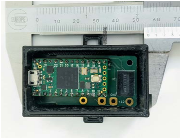
Fig. 18. Developed prototype with 3D printed case; dimensions 56x32x38 mm casing included
