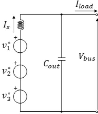
**Figure 10.** Simplified simulation model for real load profiles
