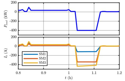
**Figure 12.** Urban ferry load cycle: detail on the battery current sharing
