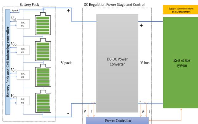
**Figure 4.** Block diagram of a monotype BESS
