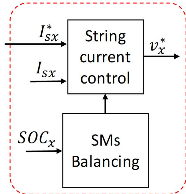
**Figure 7.** Block diagram of the string control structure
