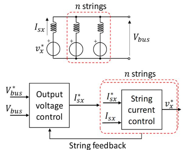
**Figure 6.** Block diagram of the HESS control structure
