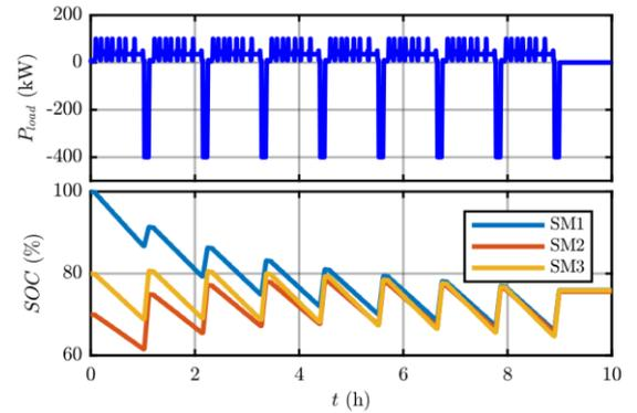
**Figure 13.** Urban ferry load cycle: SOC trend during the cycle
