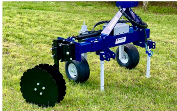
**Figure 4.** Example of a mechanical weeder.
