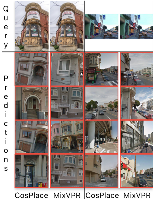
Figure 2: Examples of 2 challenging queries (top row) which present heavy viewpoint changes with respect to the database. The first and third columns are matches to the two queries obtained with CosPlace [8], while the second and fourth column are matches obtained with MixVPR [2].
