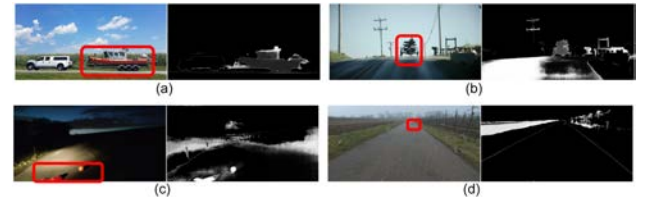
Fig. 15. Failure Cases : (a, b) Mask2Anomaly fail to segment trailer or carriage as they have a similar appearance as car or bus. Mask2Anomaly struggle to perform well in poor illumination (c) and weather conditions (d). The white region represents the anomalies that are enclosed in red boxes.
