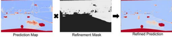
Fig. 6. Mask Refinement Illustration : To obtain the refined prediction, we multiply the prediction map with a refinement mask that is built by assigning zero anomaly scores for pixels that are categorized as “stuff”, except for the “road”. The refinement eliminates many false positives at the boundary of objects and in the background. The region to be masked is white in the refinement mask.
