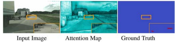
Fig. 5. Limitation of Mask-Attention : Masked-attention [14] selectively attends to foreground regions resulting in low attention scores (dark regions) for anomalies. Anomalies are in red. Best viewed with Zoom.
