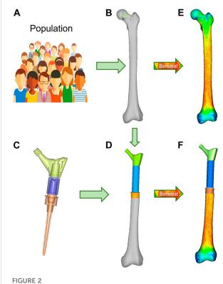
Finite element modelling workflow, described for the M-PFR configuration. From a group representative of anatomical and density variations in a population (A), the mean femur is extracted (B), and implanted with the PFR ((C), with inner details on juctions, and (D)). Both intact and implanted geometries are meshed, and CT-based material properties are assigned (E,F).
