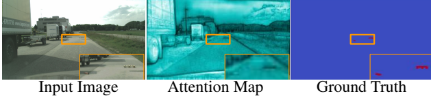
Figure 3: Limitation of Mask-Attention: Masked-attention [12] selectively attends to foreground regions resulting in low attention scores (dark regions) for anomalies. Anomalies are in red. Best viewed with zoom.
