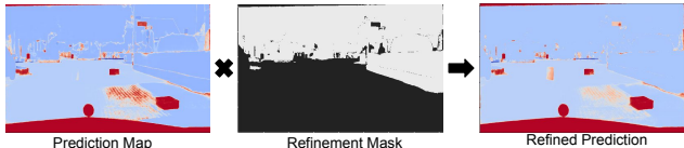
Figure 4: Mask Refinement Illustration: To obtain the refined prediction, we multiply the prediction map with a refinement mask that is built by assigning zero anomaly scores for pixels that are categorized as “stuff”, except for the “road”. The refinement eliminates many false positives at the boundary of objects and in the background. The region to be masked is white in the refinement mask.
