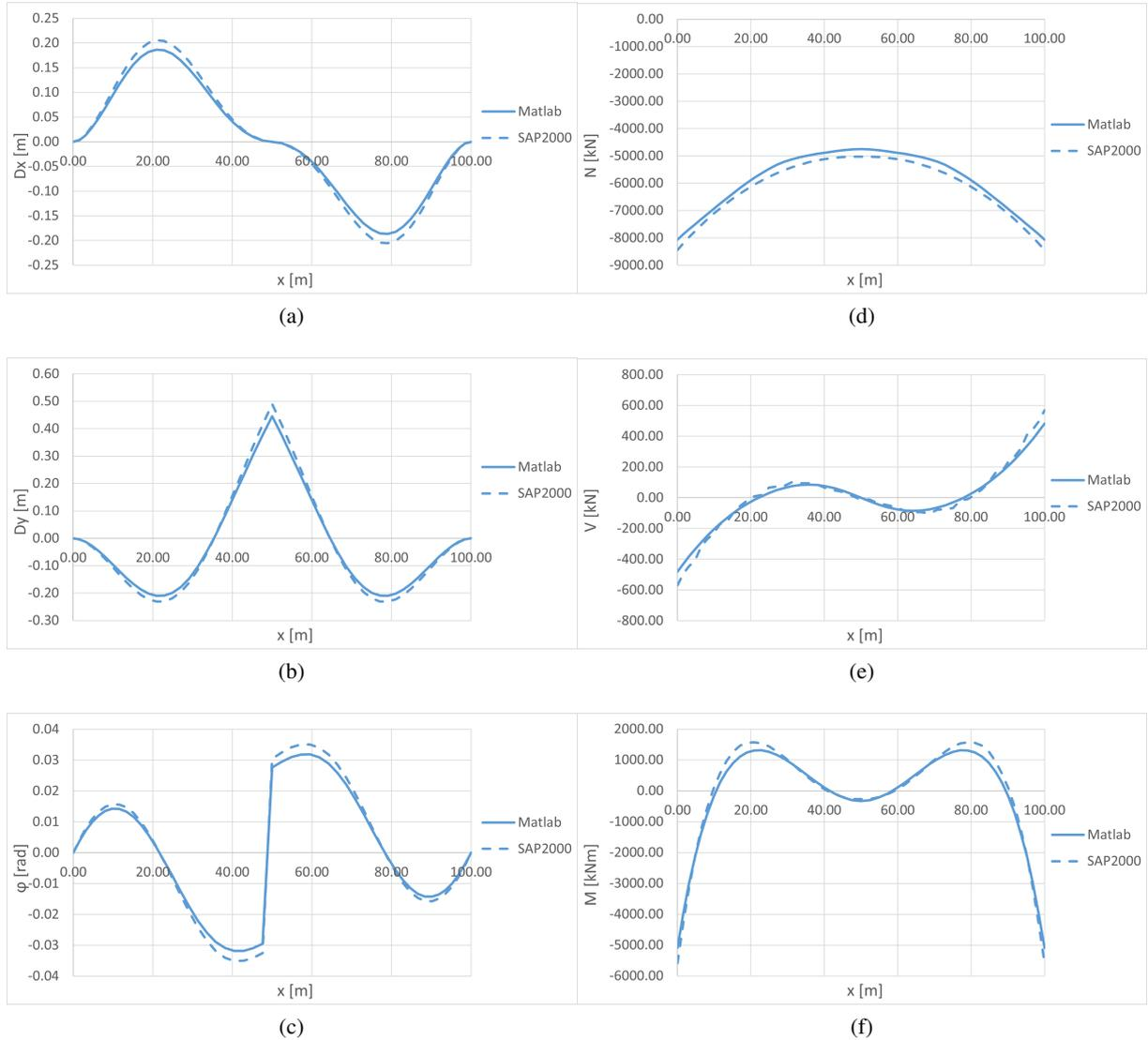
**Figure 4:** Analyses results comparison: Displacements in x-direction  $Dx$  (a), Displacements in y-direction  $Dy$  (b), Rotations  $\phi$  (c), Axial Force  $N$  (d), Shear Force  $V$  (e), Bending Moment  $M$  (f).
