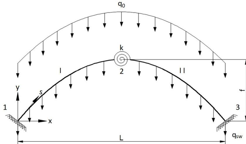
**Figure 2:** Static scheme of a fully restrained arch with a rotational hinge in the mid-span, subjected to self-weight load  $q_{sw}$  and an overload  $q_0$
