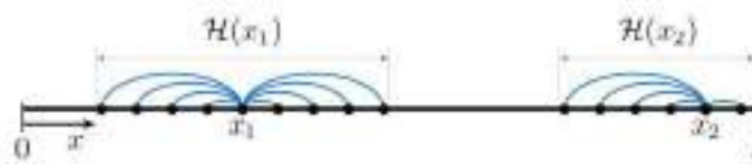
Figure 1: Example of the neighborhoods of two points ( x_1 and x_2 ) in a peridynamic body. Note that the neighborhood of point x_2 is incomplete due to the closeness with the boundary of the body, whereas the neighborhood of point x_1 in the bulk of the body is complete. The blue curved lines represent the PD bonds between points x_1 , x_2 , and their neighboring points, respectively.
