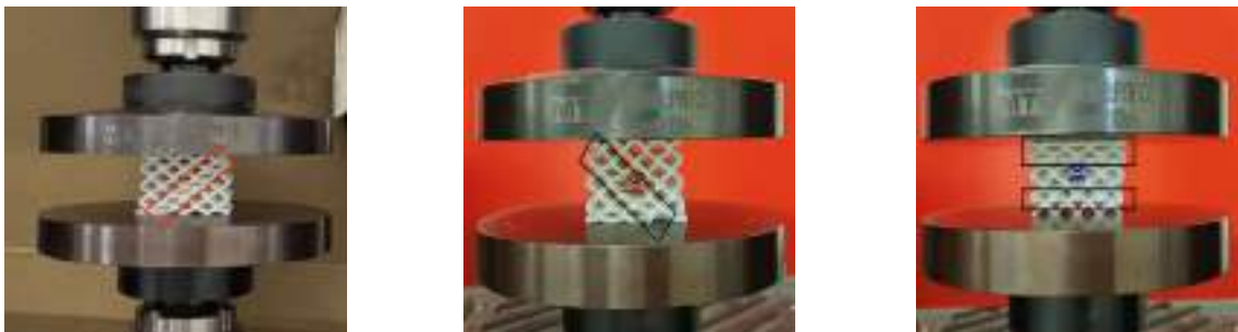
Figure 11 – Deformation modes of BCC lattice structure. Shear bands details.
