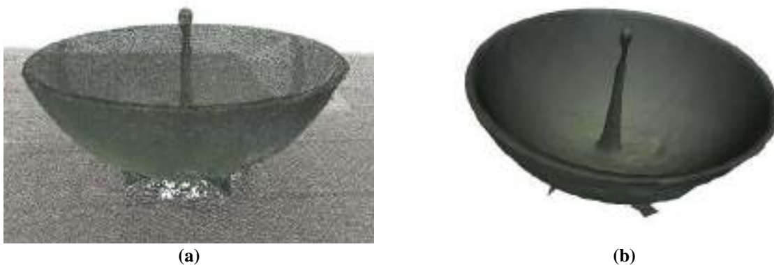
(a) (b) Figure 5 Final points cloud (a) and reconstructed mesh (b).
