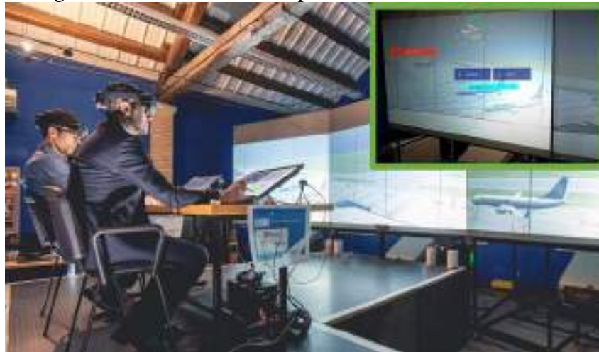
Figure 2: University of Bologna simulation and validation platform at the Virtual and Simulation Laboratory in Forlì premises. The ATCOs are provided with a realistic and consistent scenario of the out-of-the-tower view of the aerodrome onto a CAVE-like virtual environment, by wearing the ST-HMD devices the users can simultaneously see the both the AR overlays and the out-of-the-window view (personal view of the specific ATCO in the green square).
