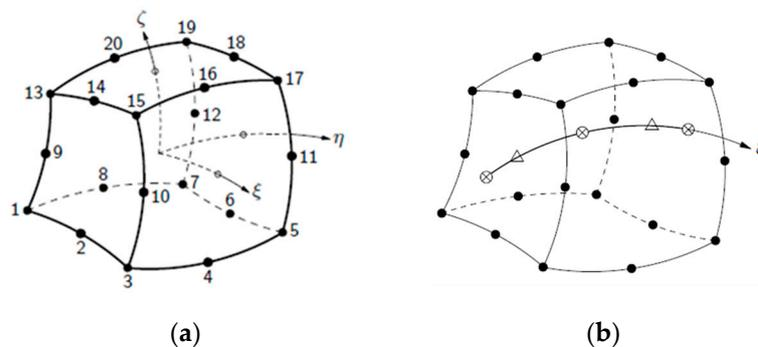
**Figure 12.** Elements used for nonlinear 3D modelling [35]. (a) A 20 nodes brick element. (b) Embedded bar element.
