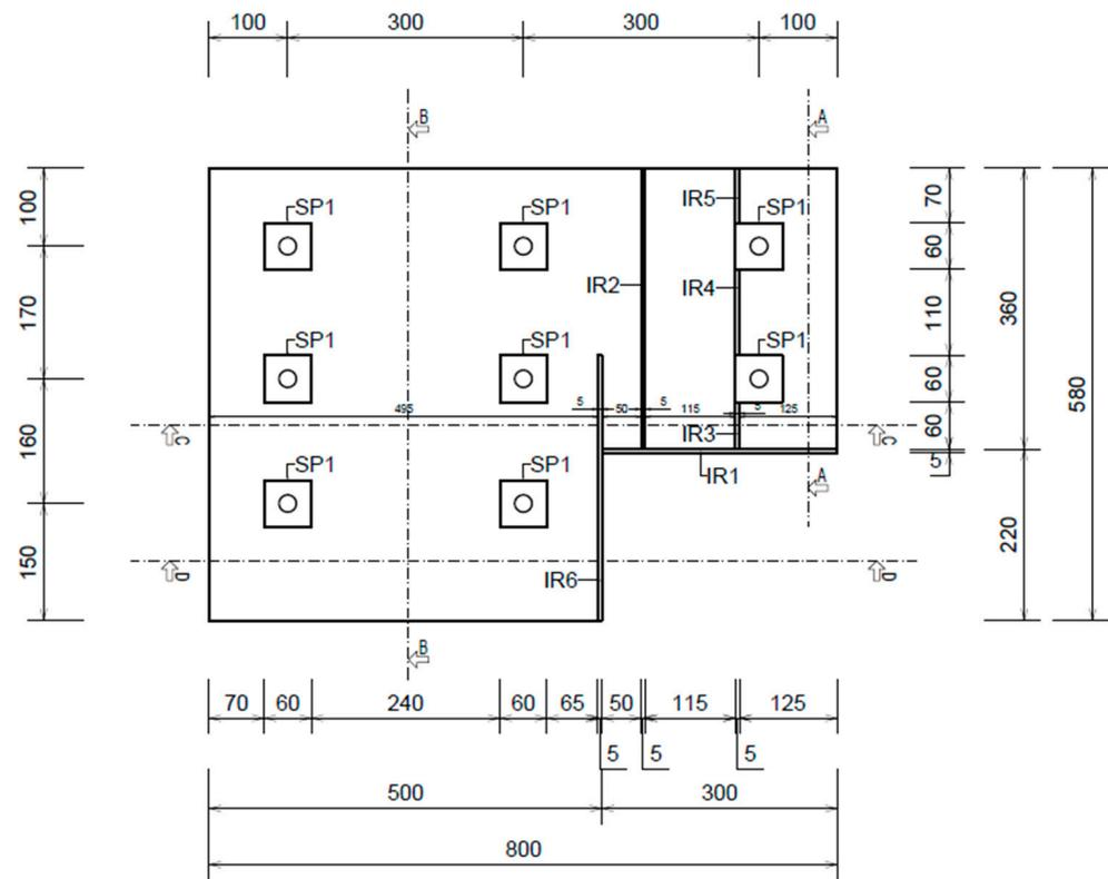
Figure 8. The geometry of the steel plates.
