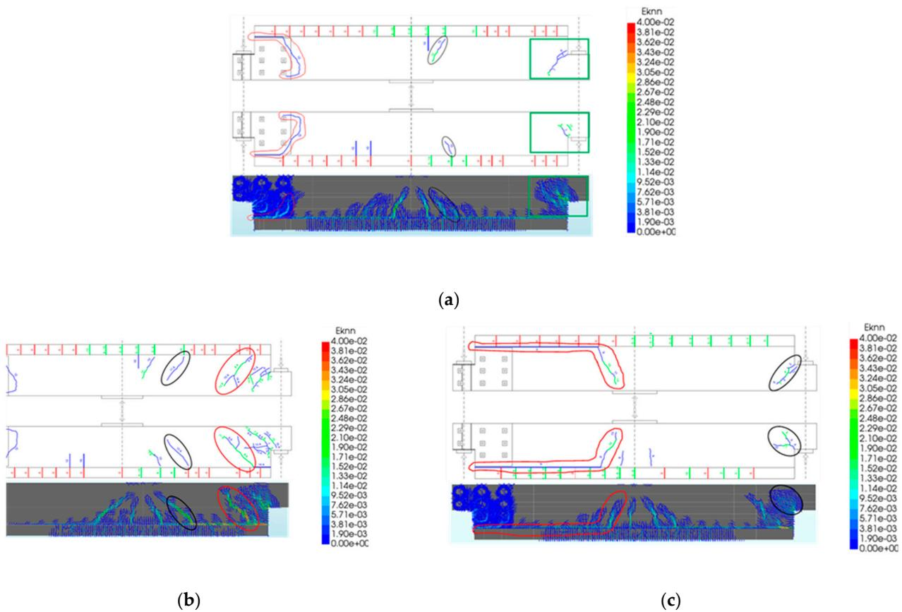
**Figure 20.** Comparison between experimental and numerical crack pattern. (a) Beam with orthogonal reinforcement in static scheme 1. (b) Beam with orthogonal reinforcement in static scheme 2. (c) Beam with inclined reinforcement in static scheme 1.
