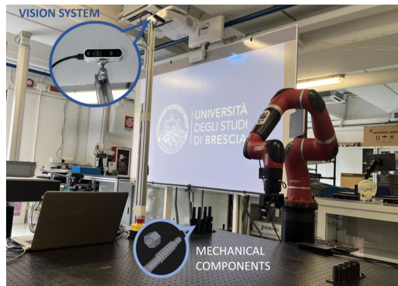
Figure 8. Experimental setup consisting of a Sawyer cobot, vision system (RealSense D435 camera), and the mechanical tools highlighted.
