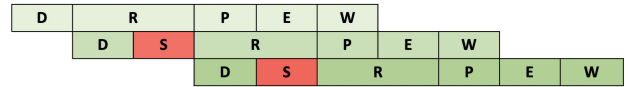
FIGURE 8. The different stages of the pipeline: [D]iscovery, [R]eading, [P]arsing, [E]laboration, [W]rite-Back. In a realistic scenario, some [S]talls might be present.
