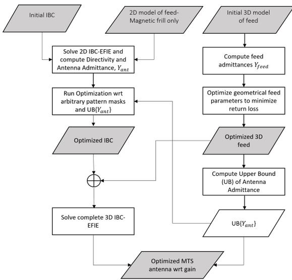
Fig. 2. Flow-chart of the accelerated design process.
