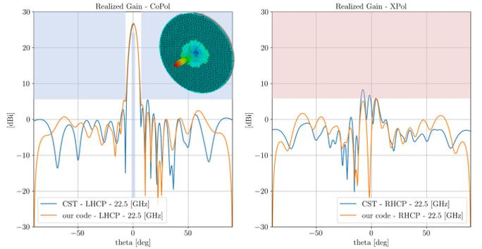
Fig. 3. Realized Gain of the metasurface antenna: co-pol (left) and x-pol (right) radiated by the antenna for  $\theta \in [-90, 90]$  and  $\phi = 0$ . Blue solid lines refer to CST simulation, orange solid lines to our code. Blue and red shaded area represent the co-polar and cross-polar pattern mask used in the optimization process, respectively.
