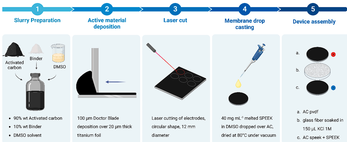
Fig. 2. Flowchart of electrodes and device production process.
