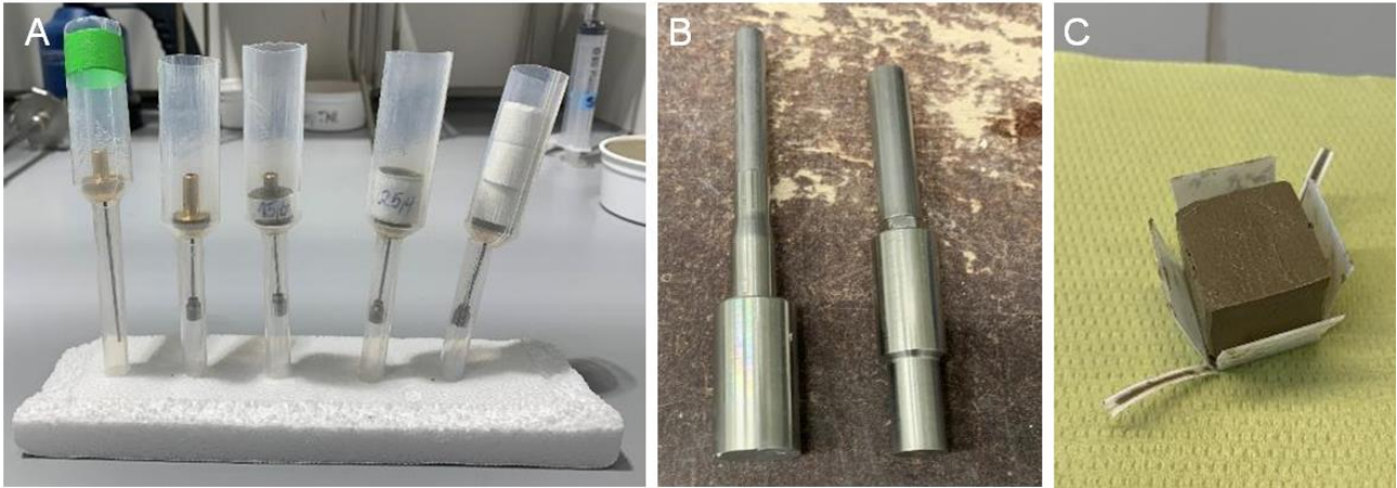
92 Fig. 1 Vicat needles for early strength (A), penetrometers (B) and a cube for the 93 compressive strength test (C).
