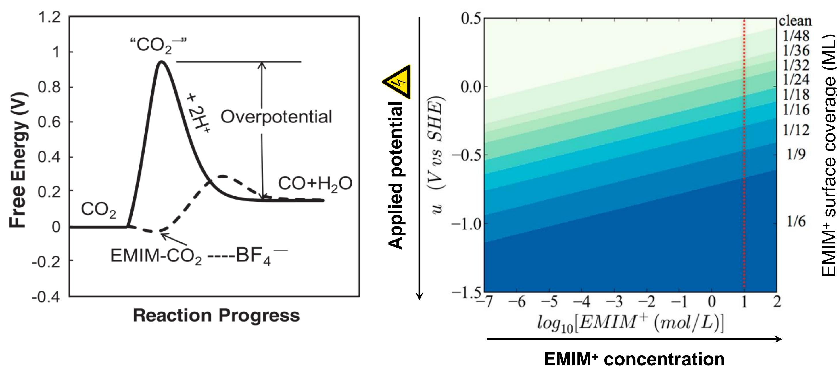
Ionic liquids promote CO<sub>2</sub> activation,<sup>2,3,4</sup> yet they can poison the surface at high concentration and negative potential.<sup>5</sup>
