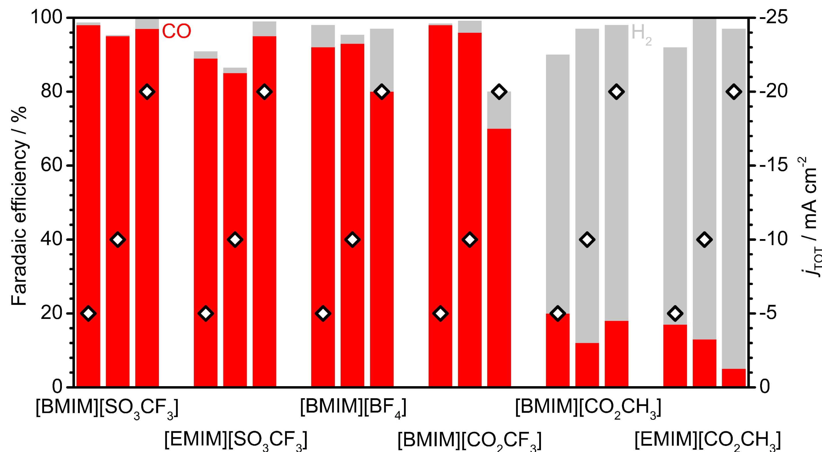
Electrochemical CO<sub>2</sub> reduction on polycrystalline silver in imidazolium-based ionic liquids.<sup>1</sup>
