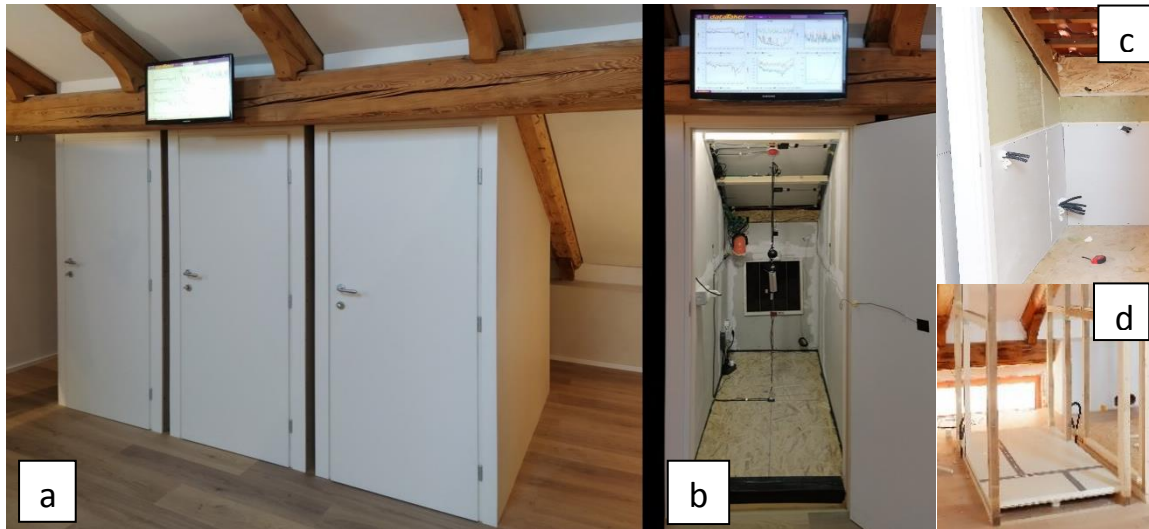
Fig. 1 a) The three test rooms; b) Internal view and sensors position; c) Construction of walls d) Construction of floors
