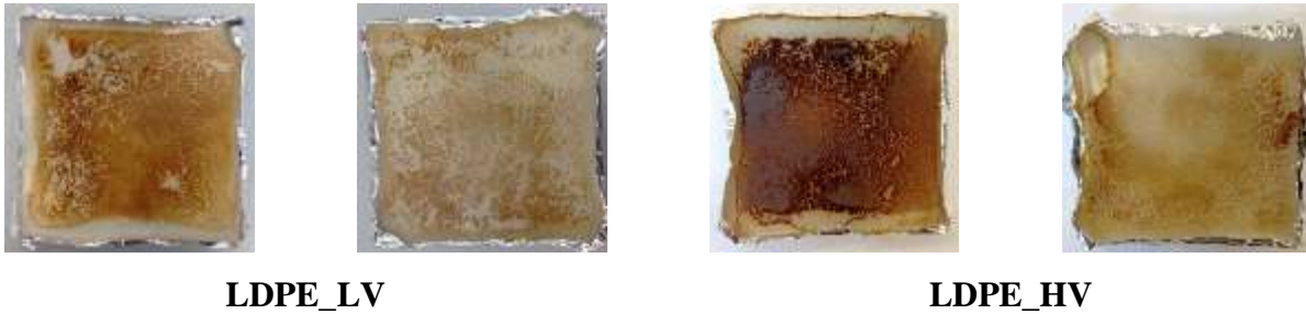
Figure 9. Appearance of the surface of specimens quenched at ignition time during cone calorimeter tests at 20 and 35 kW/m 2 .
