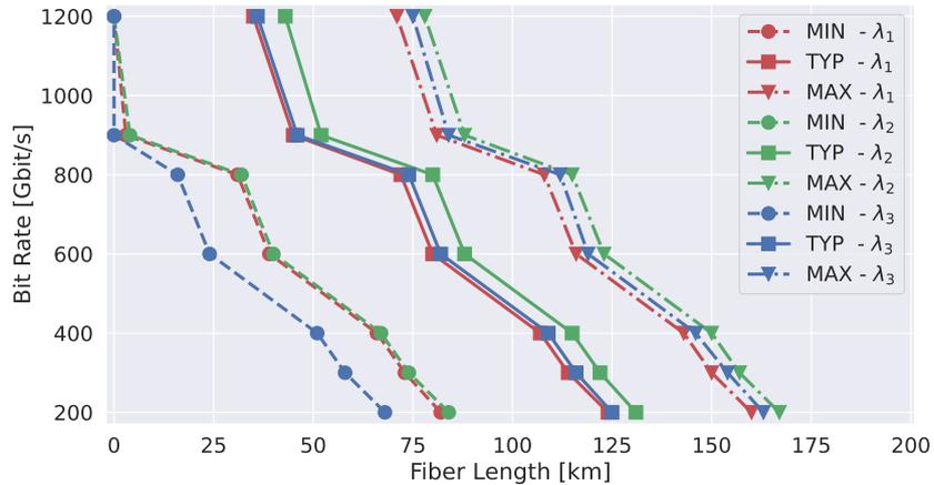
Fig. 4: Bit Rate [Gbit/s] vs. Fiber Length [km] obtained by simulation, considering three SOA operating conditions (MIN, TYP and MAX) for three wavelengths  $\lambda_{1,2,3}$  under test, at 191.5, 193.5 and 195.5 THz, respectively.
