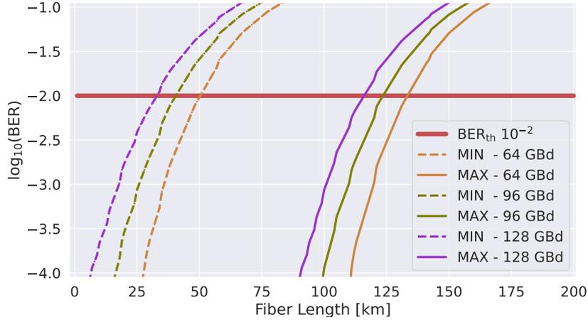
Fig. 3:  $\log_{10}(\text{Pre-FEC BER})$  vs. Fiber Length [km] curves obtained by simulation, considering two SOA operating conditions (MIN and MAX), and three symbol rates (64, 96 and 128 GBd) for a DP-16 QAM modulation format, for a channel at 193.5 THz.
