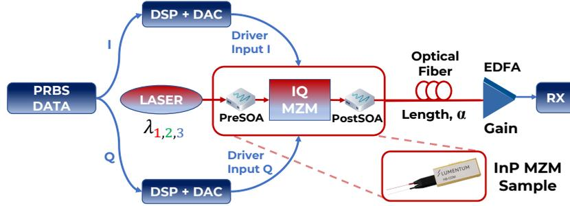
Fig. 1: Block scheme of the simulation framework.
