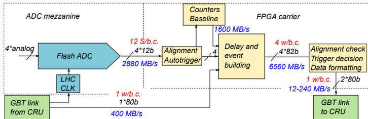
**Figure 2.** Scheme of the data flow in the FPGA firmware for a readout module. The rate of information for each link is shown as red text, in black the number of lanes \* the bus width, and in blue the data bandwidth.
