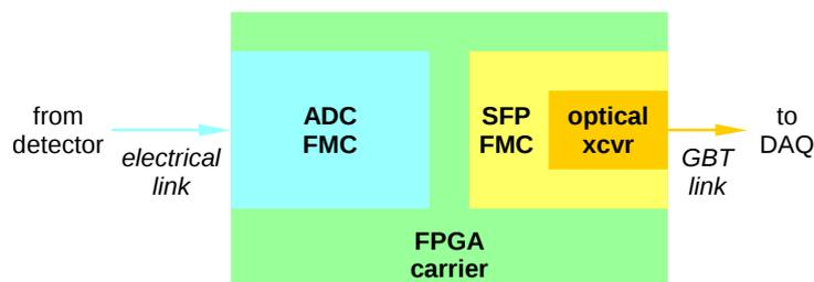
**Figure 1.** Scheme of the readout system for the ZDC upgrade. A fast digitizer in FMC format is read out by a FPGA and the portions of waveform where a signal is present are transferred to the acquisition through an optical link (GBT).
