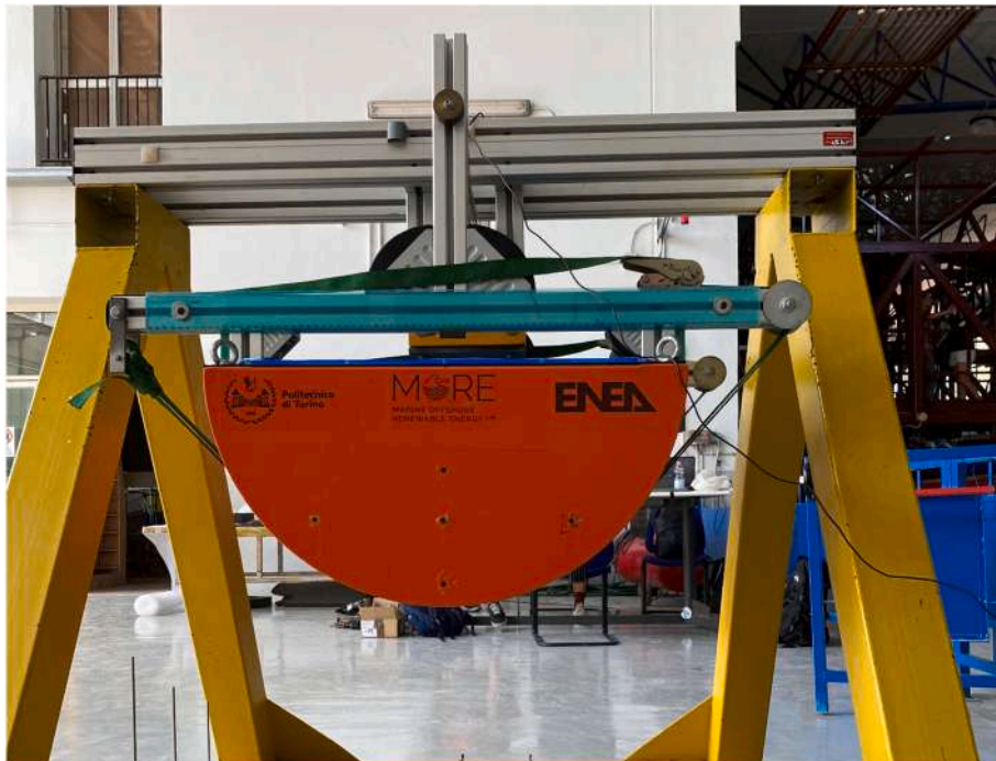
Fig. 5. PEWEC on inertial balance.
