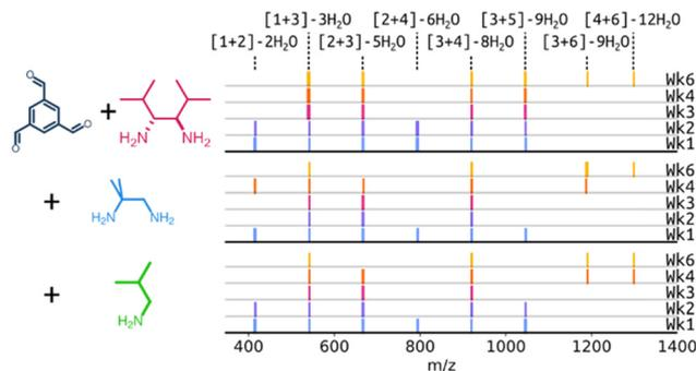
**Fig. 2** Representation of the mass spectra collected over 6 weeks for the different reaction conditions screened to investigate formation of **CC21** in  $\text{CDCl}_3$  with  $\text{NEt}_3$  at room temperature, with the observed identifiable [TFB + DMHDA] intermediates shown. Note that this does not include any information in relation to relative peak intensities in the mass spectra.
