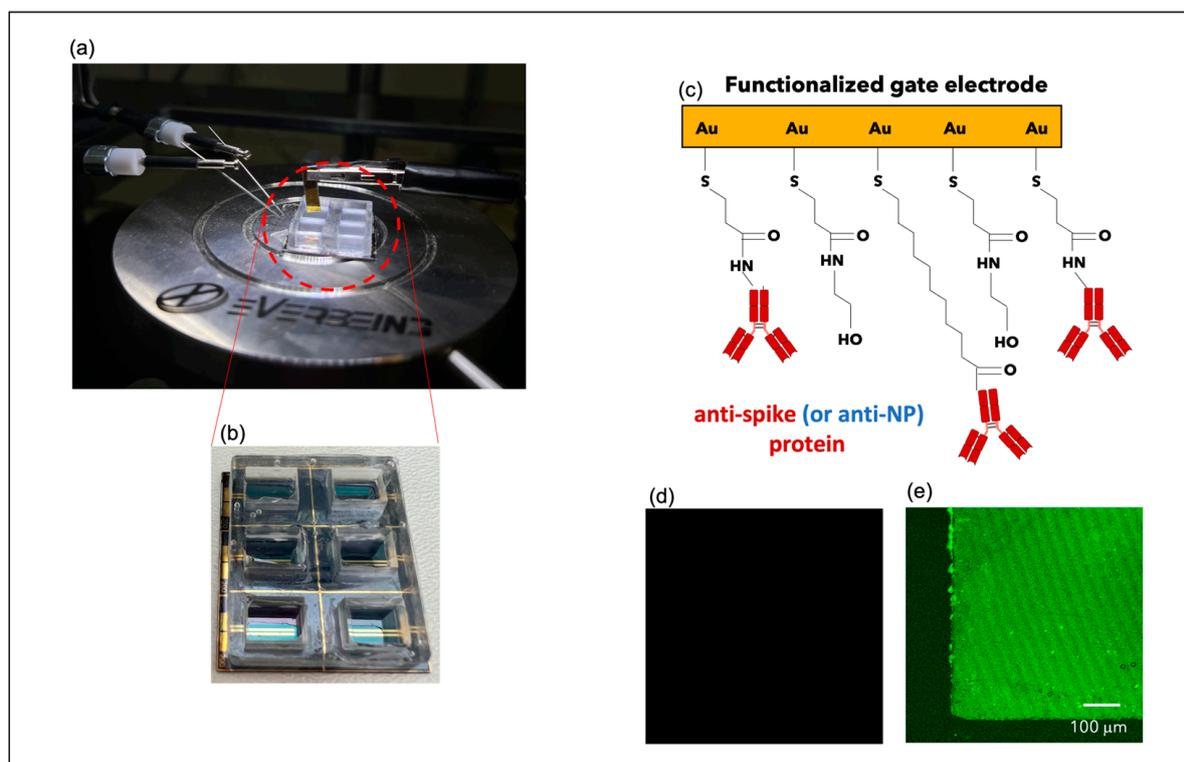
**Figure 1.** (a,b) Pictures of the layout of the employed OECT devices and of the external gate electrodes; (c) cartoon of the gate electrode functionalization; CLSM gate images before (d) and after (e) incubation with secondary antibodies conjugated to Alexa Fluor<sup>®</sup> 488 dye.
