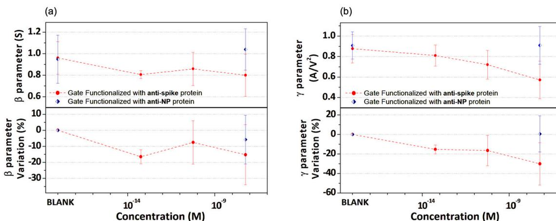
**Figure 6.**  $\beta$  and  $\gamma$  fitting parameters (top panels) and the corresponding percent variations (bottom panels) are reported in (a,b), respectively, as a function of the spike-RBD protein concentration for gate electrodes functionalized with spike and nucleocapsid antibodies.
