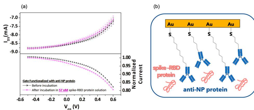
**Figure 4.** (a) Transfer curves (top panel) and normalized transfer curves with respect to the  $I_{DS}$  current recorded at  $V_{GS} = -0.5$  V (bottom panel) as a function of  $V_{GS}$  by using a functionalized gate with nucleocapside (NP) antibody before and after incubation in 57 nanomolar spike-RBD protein solution; (b) cartoon of the anti-NP protein and spike-RBD protein unbound configuration.
