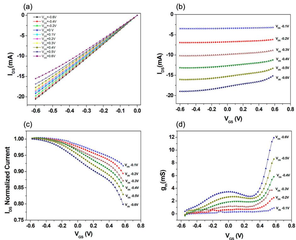
**Figure 2.** (a) Output curves reporting  $I_{DS}$  as a function of  $V_{DS}$  and applying  $V_{GS}$  between  $-0.6$  and  $0.6$  V; (b) OECT transfer curves and (c) normalized transfer curves, with respect to the  $I_{DS}$  current at  $V_{GS} = -0.6$  V, measured as a function of  $V_{GS}$  with  $V_{DS}$  ranging from  $-0.6$  to  $-0.1$  V; (d) transconductance  $g_m$  as a function of  $V_{GS}$  with  $V_{DS}$  ranging between  $0.1$  and  $-0.6$  V.
