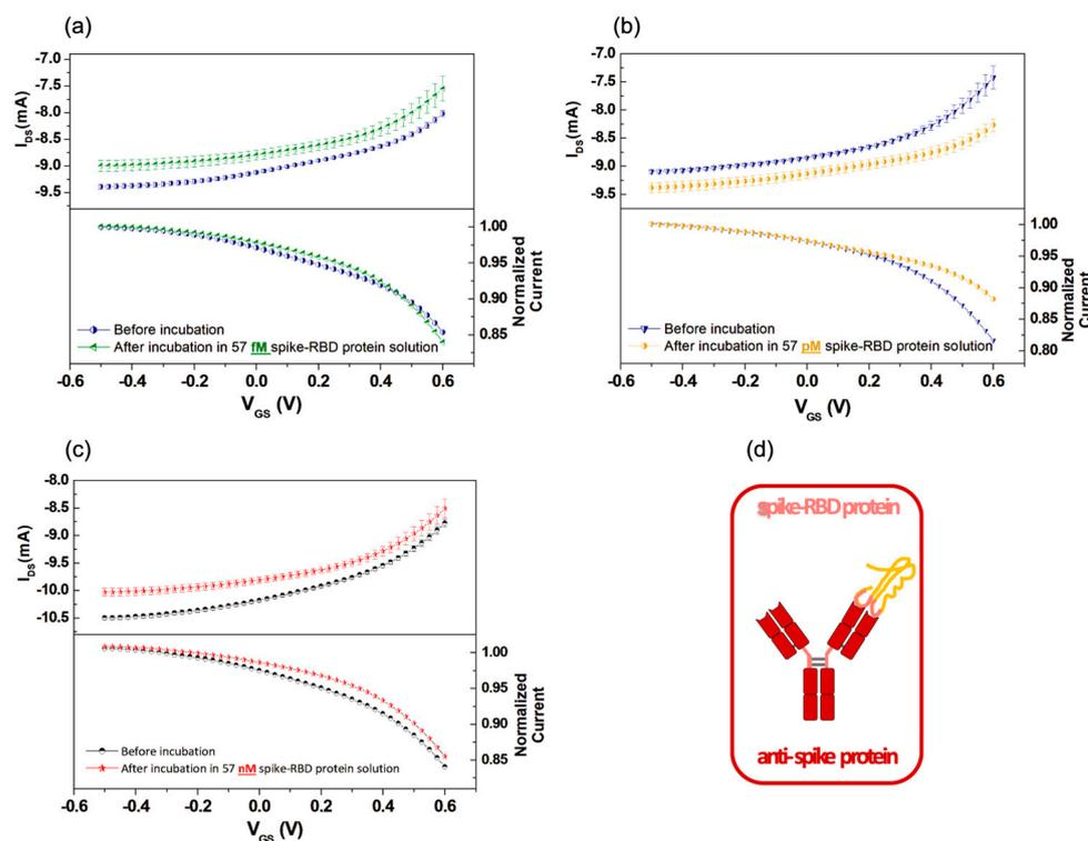
**Figure 3.** Transfer curves (top panels) and normalized transfer curves with respect to the  $I_{DS}$  current recorded at  $V_{GS} = -0.5$  V (bottom panels) measured as a function of  $V_{GS}$  by using a functionalized gate with anti-spike protein before incubation and after incubation in solutions with (a) 57 femtomolar (fM) spike-RBD protein; (b) 57 picomolar (pM) spike-RBD protein; (c) 57 nanomolar (nM) spike-RBD protein; (d) cartoon reporting the spike antibody–antigen binding event.
